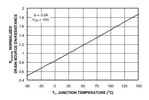
Figure 3. On-Resistance Variation with Temperature.
