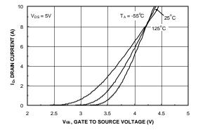
Figure 5. Transfer Characteristics.
