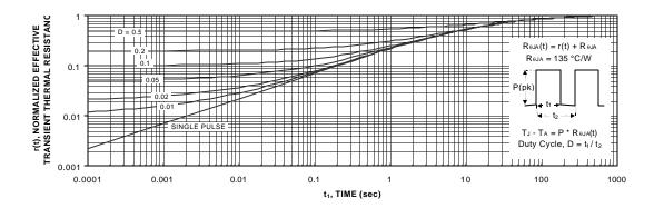
Figure 11. Transient Thermal Response Curve.
