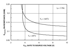
Figure 4. On-Resistance Variation with Gate-to-Source Voltage.
