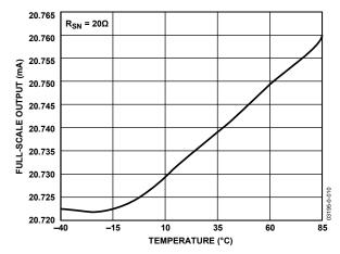
Figure 9. Full-Scale Output vs. Temperature
