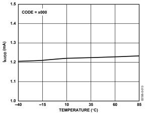
Figure 12. AVDD Supply Current (I<sub>AVDD</sub>) vs. Temperature
