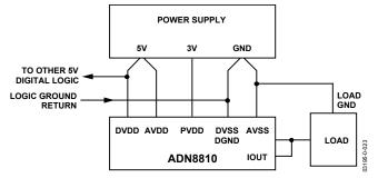
Figure 23. Star Supply and Ground Technique
