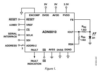
Noise and digital feedthrough are kept low to ensure low jitter operation for laser diode applications. Full-scale and scaled output currents are given in Equation 1 and Equation 2, respectively.
