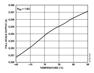
Figure 8. Full-Scale Output vs. Temperature
