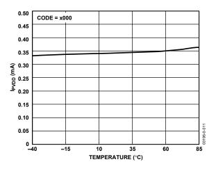
Figure 10. PVDD Supply Current (I<sub>PVDD</sub>) vs. Temperature
