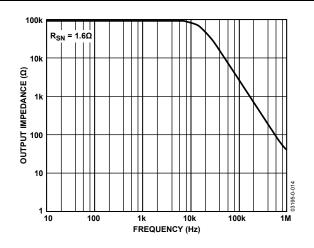
Figure 13. Output Impedance vs. Frequency
