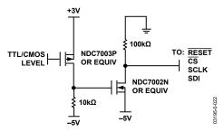
Figure 22. Level Shifting TTL/CMOS Logic
