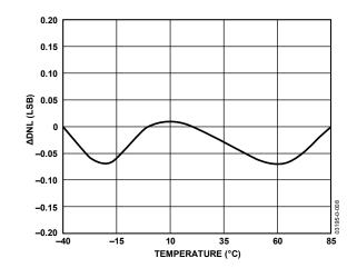
Figure 7. ΔDNL vs. Temperature
