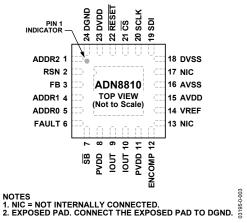
Figure 3. Pin Configuration
