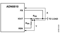
Figure 24. Use Identical Trace Lengths for Sense Resistors
