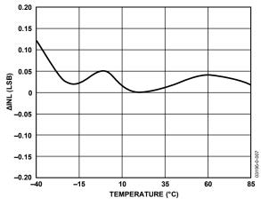
Figure 6. ΔINL vs. Temperature
