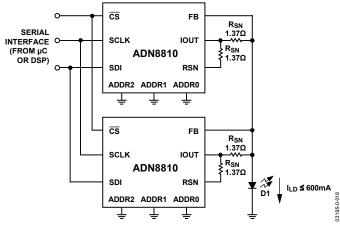
Figure 18. Using Multiple Devices for Additional Output Current
