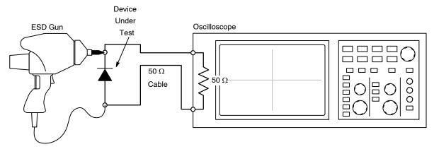
Figure 4. Diagram of ESD Clamping Voltage Test Setup
