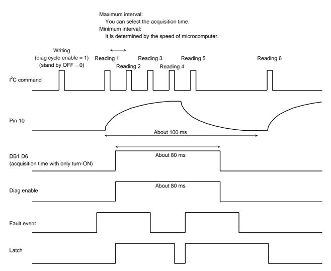
The turn ON diagnostic acquisition time is determined by the ripple filter capacitance C2 and the equivalent internal resistance Rr as below expression.
