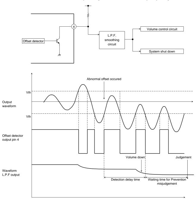
Figure 9 Hardware Output Offset Detection
