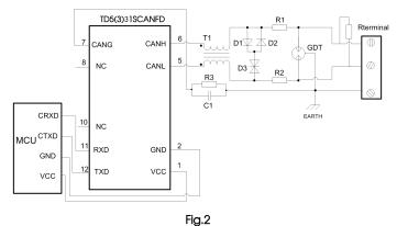
Note: Ground shield of twisted wire pair reliably.
