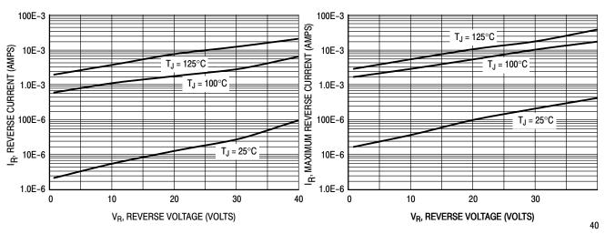
**Figure 3. Typical Reverse Current**
