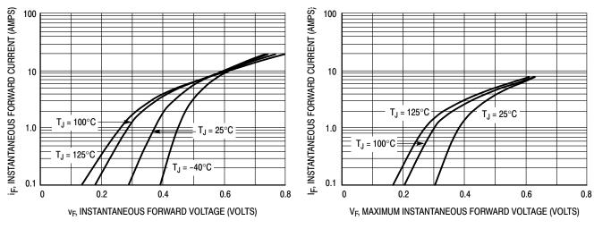
Figure 1. Typical Forward Voltage
