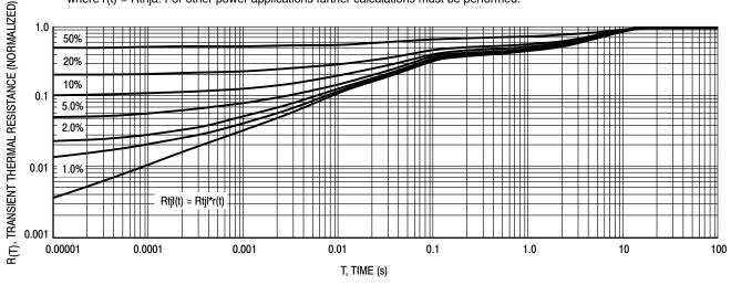
Figure 9. Thermal Response Junction to Lead R(T), TRANSIENT THERMAL RESISTANCE (NORMALIZED) 1.0 50% 0.1 10% 5.0% 2.0% 0.01 1.0% Rtjl(t) = Rtjl\*r(t)0.001 0.00001 0.0001 0.001 0.01 0.1 1.0 10 100 1,000 T, TIME (s)
