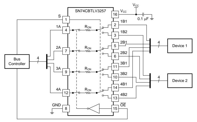
Figure 2. Typical Application of the SN74CBTLV3257
