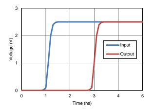
Figure 3. Propagation Delay (tpd) Simulation Result at V<sub>CC</sub> = 2.5 V
