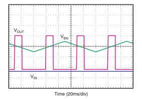
Figure 28. Enable Pin Positive and Negative Threshold
