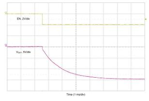
Figure 30. Start-up With a Feed-Forward Capacitor
