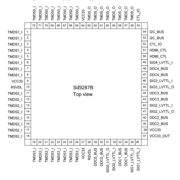
TMDS0/1/2/3\_I-- TMDS Input Port-Specific Signals
