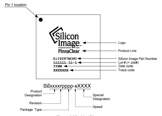
Figure 4. Marking Diagram
