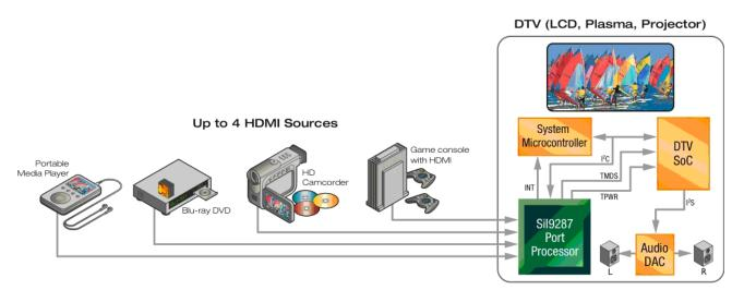
Figure 1. Typical Application of SiI9287B HDMI Port Processor
