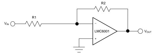
Figure 22. Typical Application Schematic, LMC6001
