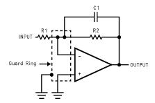
Figure 26. Inverting Amplifier
