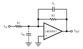
Figure 19. Cancelling the Effect of Input Capacitance
