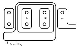
Figure 30. Examples Of Guard Ring In PCB Layout
