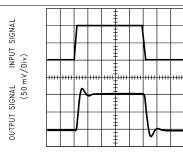
Figure 16. Noninverting Small Signal Pulse Response
