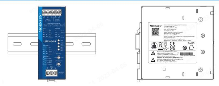
Note: Keep the following installation clearances: 20mm on top, 20mm on the bottom, 5mm on the left and right sides are recommended when the device is loaded permanently with more than 50% of the rated power. Increase this clearance to 15mm in case the adjacent device is a heat source (e.g. another power supply).
