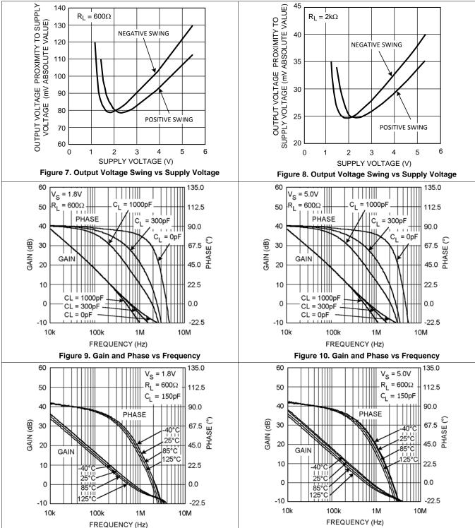
Figure 11. Gain and Phase vs Frequency
