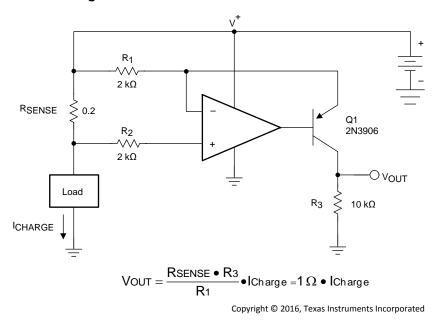
Figure 33. High-Side, Current-Sensing Schematic
