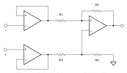
Figure 32. Rail-to-Rail Instrumentation Amplifier
