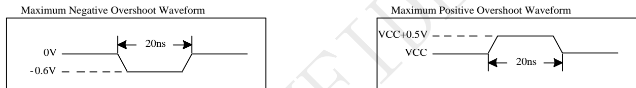
Figure 5-1 Maximum Overshoot Waveform
