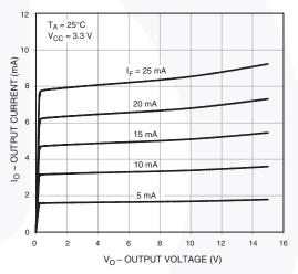
Figure 6. Output Current vs. Output Voltage
