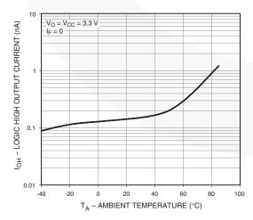
Figure 7. Logic High Output Current vs. Ambient Temperature
