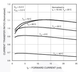
Figure 4. Current Transfer Ratio vs. Forward Current
