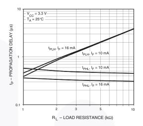
Figure 10. Propagation Delay vs. Load Resistance
