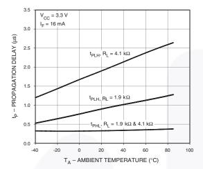
Figure 9. Propagation Delay vs. Ambient Temperature
