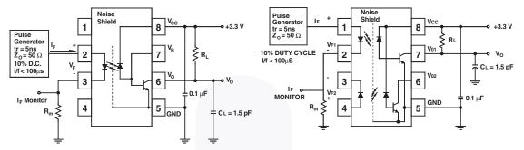
Test Circuit for FOD050L
