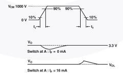
Figure 12. Common Mode Immunity Test Circuit
