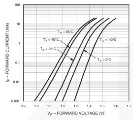
Figure 3. LED Forward Current vs. Forward Voltage
