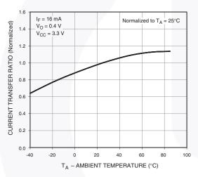
Figure 5. Current Transfer Ratio vs. Ambient Temperature
