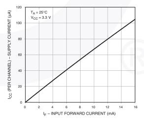
Figure 8. Supply Current vs. Input Forward Current
