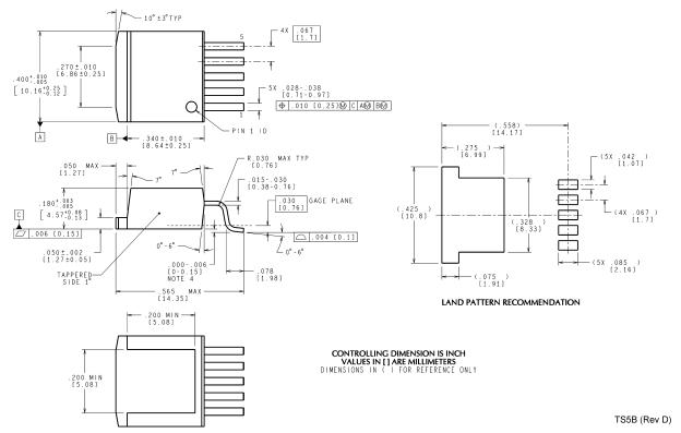
TO263 5-Lead, Molded, Surface Mount Package (TO263-5)
