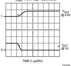
Load Transient Response  $C_{IN} = 4 \times 10 \mu F$  CERAMIC  $C_{OUT} = 3 \times 10 \mu F$  CERAMIC
