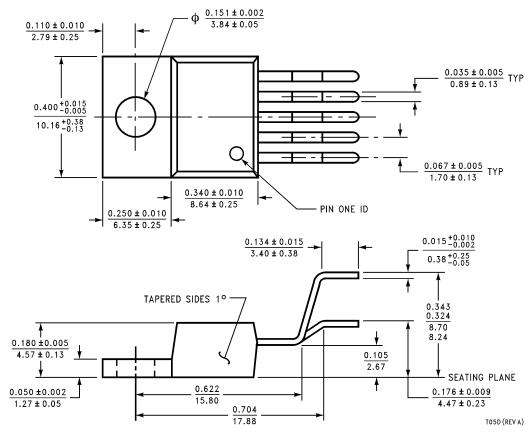
TO220 5-lead, Molded, Stagger Bend Package (TO220-5)
