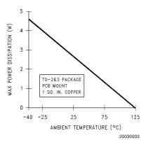
FIGURE 6. Maximum power dissipation vs ambient temperature for TO-263 package
