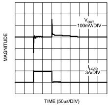
Load Transient Response  $C_{IN} = 4 \times 10 \mu F$  CERAMIC  $C_{OUT} = 3 \times 10 \mu F$  CERAMIC
