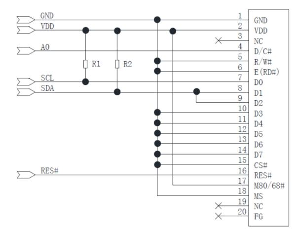
Pin connected to MCU interface: SDA, SCL, SA0, RES#.
