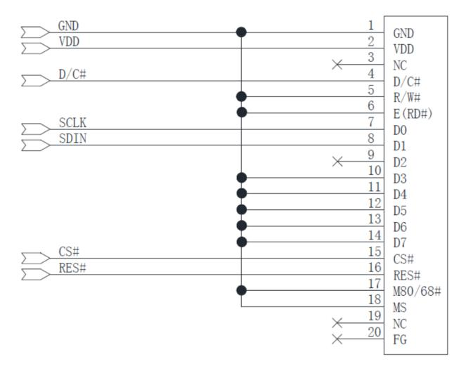
Pin connected to MCU interface: SDIN, SCLK, RES#, D/C#, CS#.
