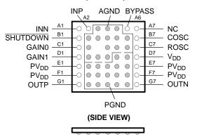
NC – No internal connection, still requires a pad for the ball.NOTE: The shaded terminals are used for thermal connections to the ground plane.
