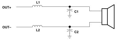
Figure 11. Class-D Output Filter
