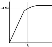
The value of  $C_i$  is important because it directly affects the bass (low frequency) performance of the circuit. Consider the example where  $Z_i$  is 20 k $\Omega$  and the specification calls for a flat bass response down to 80 Hz. Equation 5 is reconfigured as Equation 6.
