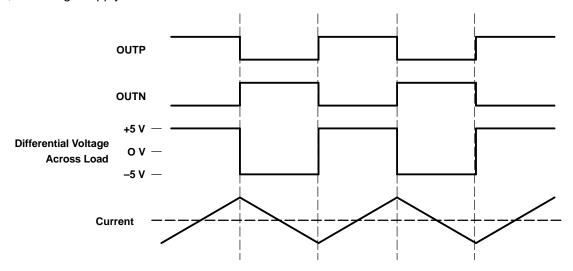
Figure 9. Traditional Class-D Modulation Scheme Output Voltage and Current Waveforms Into an Inductive Load With No Input
