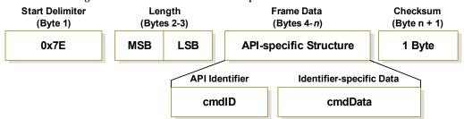
The cmdID frame (API-identifier) indicates which API messages will be contained in the cmdData frame (Identifier-specific data). Refer to the sections that follow for more information regarding the supported API types. Note that multi-byte values are sent big endian.
