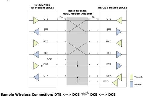
Figure 2-04. Typical wireless link between DTE and DCE devices
