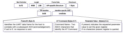
Figure 4-08. Example: API frames when reading the DL parameter value of the modem.
