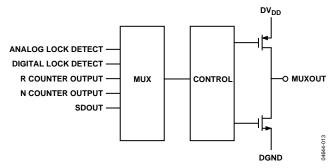
Figure 13. MUXOUT Circuit
