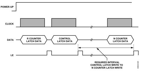
Figure 16. ADF4360-0 Power-Up Timing
