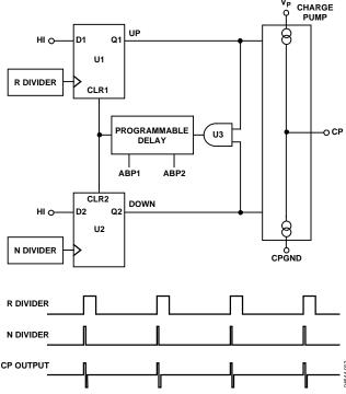
Figure 12. PFD Simplified Schematic and Timing (In Lock)
