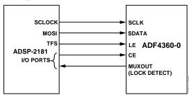
Figure 19. ADSP-2181 to ADF4360-0 Interface
