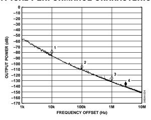
Figure 4. Open-Loop VCO Phase Noise
