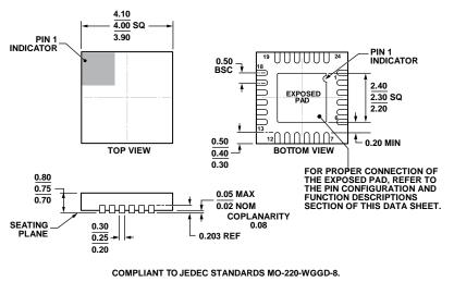
Figure 23. 24-Lead Lead Frame Chip Scale Package [LFCSP] 4 mm × 4 mm Body and 0.75 mm Package Height (CP-24-14) Dimensions shown in millimeters
