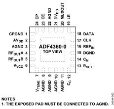
Figure 3. Pin Configuration
