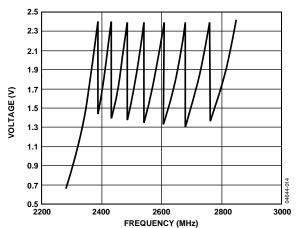
Figure 14. Frequency vs. V<sub>TUNE</sub>, ADF4360-0
