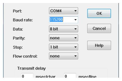
Figure 3. Serial Port Settings
