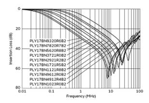
Common Mode Insertion Loss-Frequency Characteristics
