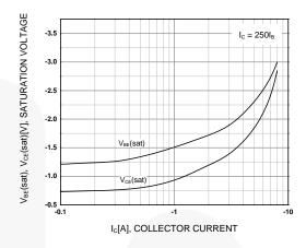
Figure 2. Base-Emitter Saturation Voltage and Collector-Emitter Saturation Voltage
