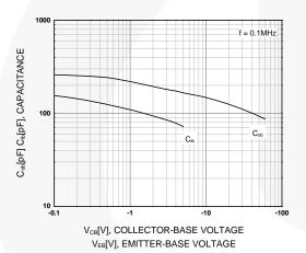
Figure 3. Output and Input Capacitance vs. Reverse Voltage
