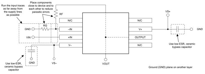
Figure 33. Operational Amplifier Board Layout for Noninverting Configuration
