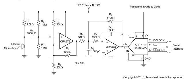
Figure 30. The OPA2373 as a Speech Bypass-Filtered Data Acquisition System
