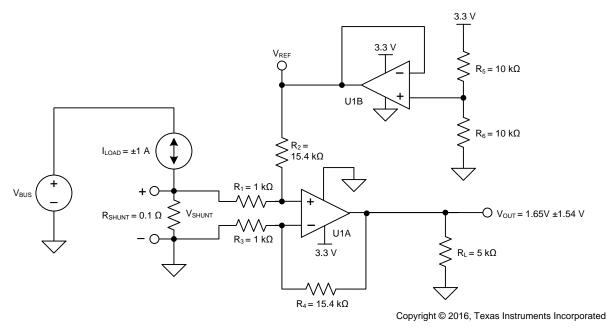
Figure 27. Single-Supply, Low-Side, Bidirectional Current-Sensing Solution
