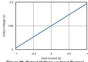
Figure 28. Output Voltage vs Input Current
