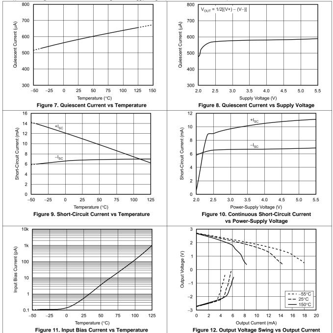
At  $T_A = 25^{\circ}$ C,  $R_L = 10 \text{ k}\Omega$  connected to  $V_S/2$ , and  $V_{OUT} = V_S/2$  (unless otherwise noted)
