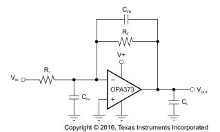
Figure 25. Improving Capacitive Load Drive
