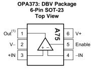
(1) Pin 1 of the 6-pin SOT-23 is determined by orienting the package marking as shown.
