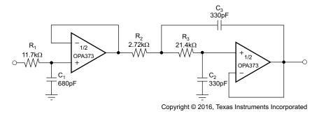
Figure 32. Three-Pole, Sallen-Key, Butterworth Low-Pass Filter
