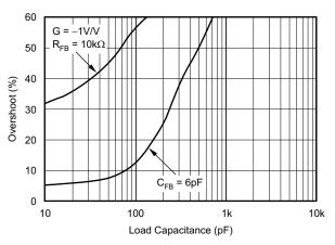
Figure 26. Improving Capacitive Load Drive
