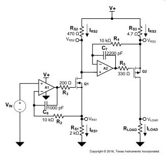
Figure 44. High-Side Voltage-to-Current (V-I) Converter
