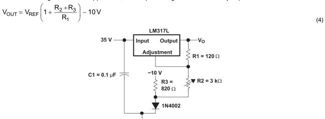
Figure 4. 0-V to 30-V Regulator Circuit
