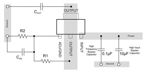
Figure 11. Layout Diagram
