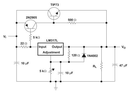
Figure 10. High-Current Adjustable Regulator
