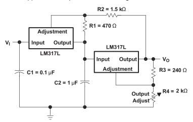
Figure 6. Tracking Preregulator Circuit
