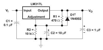
Figure 3. Regulator Circuit With Improved Ripple Rejection
