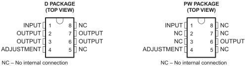
NC - No internal connection OUTPUT terminals are all internally connected.
