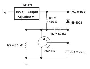
Figure 7. Slow-Turn On 15-V Regulator Circuit
