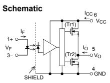
A 0.1-µF bypass capacitor must be connected between pins 6 and 4. (See Note 6.)
