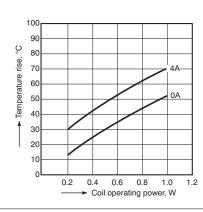
4.-(2) Coil temperature rise Tested Sample: S4-24V, 4 Form A
