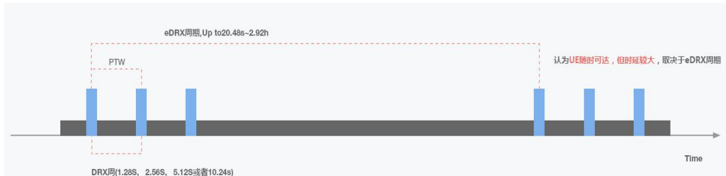
Figure 3-13 eDRX power saving technology
