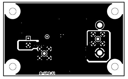
Figure 17. LM5008A Evaluation Board Bottom Layer
