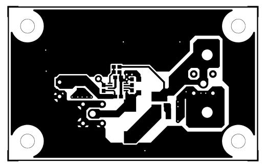
Figure 16. LM5008A Evaluation Board Top Layer
