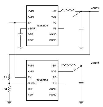
Figure 7. Sequence for Ratiometric and Simultaneous Startup
