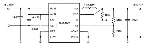
Figure 43. 2.5-V / 3-A Power Supply
