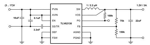
Figure 46. 1.2-V / 3-A Power Supply
