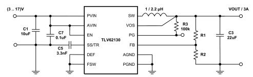
Figure 5. 3-A Step-Down Converter
