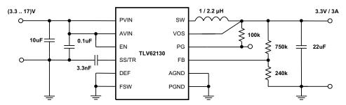
Figure 42. 3.3-V / 3-A Power Supply
