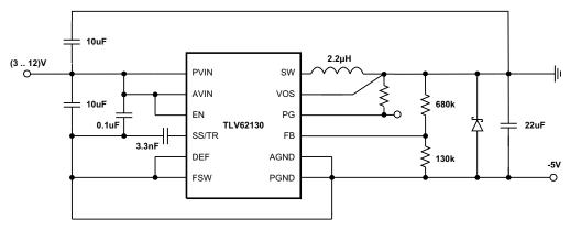
Figure 40. -5 V Inverting Power Supply
