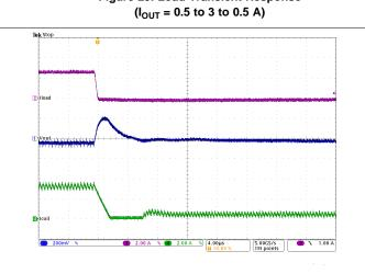
Figure 31. Load Transient Response of Figure 29, Falling Edge
