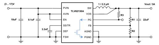
Figure 39. Discharge Vout Through PG Pin With TLV62130A
