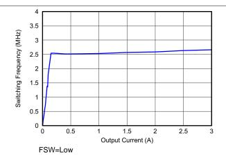
Figure 22. Switching Frequency
