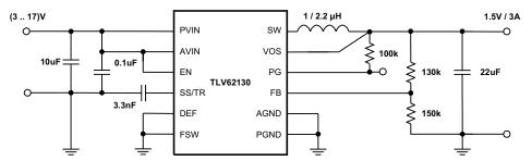
Figure 45. 1.5-V / 3-A Power Supply
