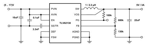
Figure 41. 5-V / 3-A Power Supply
