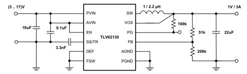
Figure 47. 1-V / 3-A Power Supply
