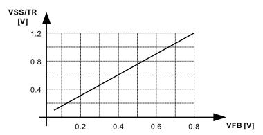
Figure 6. Voltage Tracking Relationship
