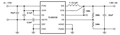
Figure 44. 1.8-V / 3-A Power Supply
