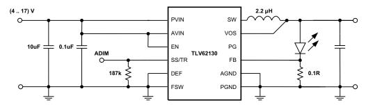
Figure 38. 3 A Single LED Power Supply
