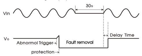
In addition, it can be quickly restarted by the PS\_ON signal:
