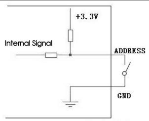
The internal pull-up resistance value of the power module is  $10k\,\Omega$ , and the external impedance can be matched according to the actual application to meet the high and low voltage range.
