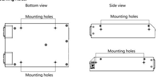
Note: The fan panel cannot be blocked by other objects, and a distance of at least 20mm must be maintained, otherwise it will affect the heat dissipation and performance of the power module.
