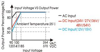
Note: With an AC input voltage between 90-100VAC and a DC input between 120-185VDC the output power must be derated as per the temperature derating curves.
