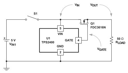
Figure 10. Output Turnon Response Test Circuit
