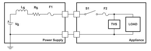
Figure 14. Load Protection Using Transient Voltage Suppressor Clamps
