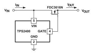
Figure 13. Application Diagram
