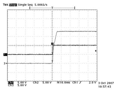
Figure 18. Circuit Start-Up With VIN = 5 V
