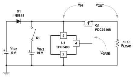
Figure 12. Output Turnoff Response Test Circuit
