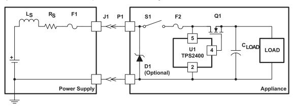
Figure 17. Turnon Voltage Slew Rate Control Using the TPS2400
