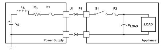
Figure 16. Power-Supply Output Resistance and Inductance Circuit Model
