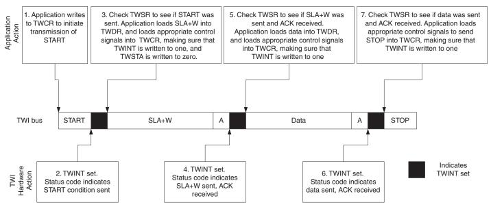
1. The first step in a TWI transmission is to transmit a START condition. This is done by writing a specific value into TWCR, instructing the TWI hardware to transmit a START condition. Which value to write is described later on. However, it is important that the TWINT bit is set in the value written. Writing a one to TWINT clears the flag. The TWI will
