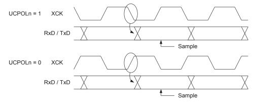
The UCPOLn bit UCRSnC selects which XCK clock edge is used for data sampling and which is used for data change. As Figure 20-3 shows, when UCPOLn is zero the data will be changed at rising XCK edge and sampled at falling XCK edge. If UCPOLn is set, the data will be changed at falling XCK edge and sampled at rising XCK edge.
