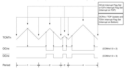
The Timer/Counter Overflow Flag (TOVn) is set at the same timer clock cycle as the OCRnx Registers are updated with the double buffer value (at BOTTOM). When either OCRnA or ICRn is used for defining the TOP value, the OCnA or ICFn flag set when TCNTn has reached TOP. The interrupt flags can then be used to generate an interrupt each time the counter reaches the TOP or BOTTOM value.
