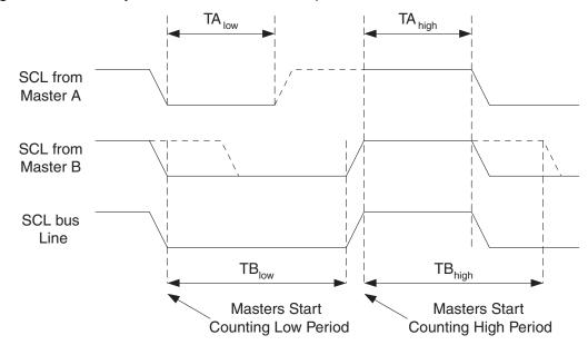
Figure 21-8. SCL Synchronization between Multiple Masters
