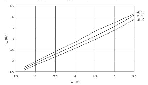
Figure 29-4. Active Supply Current vs. V<sub>CC</sub> (Internal RC Oscillator, 2 MHz)
