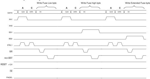
Figure 27-5. Programming the FUSES Waveforms
