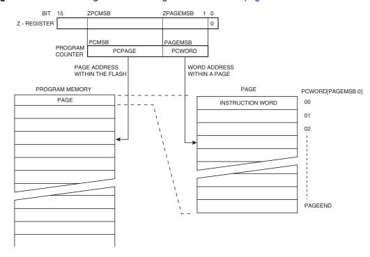
Figure 26-3. Addressing the Flash during SPM<sup>(1)</sup>Table 2 on page 287
