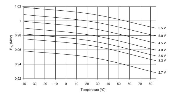
Figure 29-40. Calibrated 1 MHz RC Oscillator Frequency vs. Temperature
