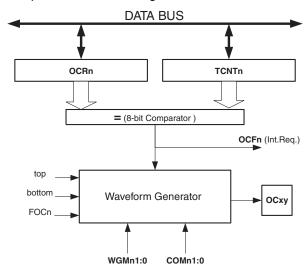
Figure 14-3. Output Compare Unit, Block Diagram
