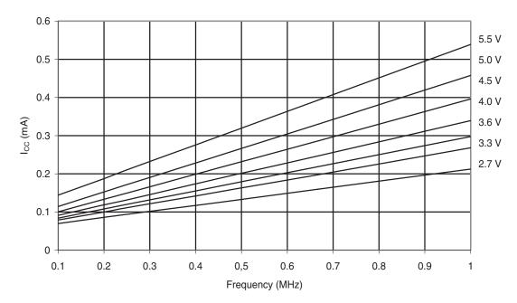
Figure 29-9. Idle Supply Current vs. Frequency (1 - 16 MHz)
