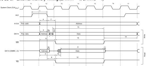
Figure 28-9. External Memory Timing (SRWn1 = 1, SRWn0 = 1)<sup>(1)</sup>
