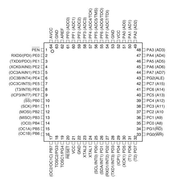
Note: The bottom pad under the QFN/MLF package should be soldered to ground.
