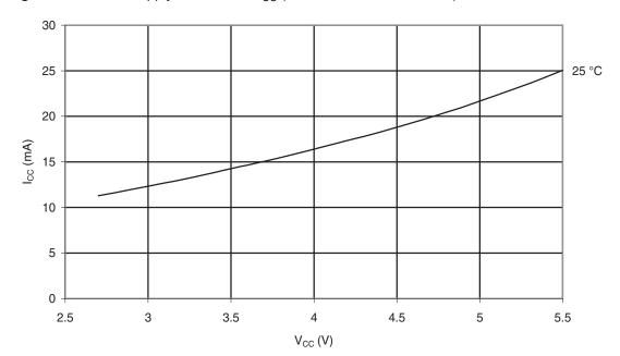
Figure 29-14. Idle Supply Current vs.  $V_{\rm CC}$  (32 kHz External Oscillator)
