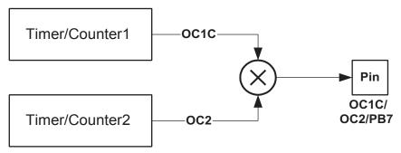
When the modulator is enabled, the two Output Compare channels are modulated together as shown in the block diagram (Figure 18-1).
