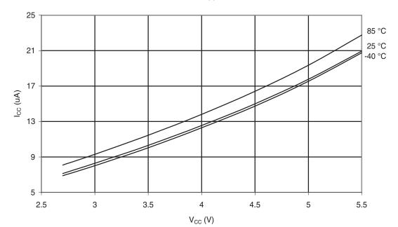
Figure 29-16. Power-Down Supply Current vs.  $V_{\text{CC}}$  (Watchdog Timer Enabled)
