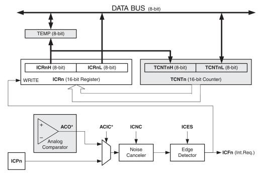
Note: 1. The Analog Comparator Output (ACO) can only trigger the Timer/Counter1 ICP – not Timer/Counter3.
