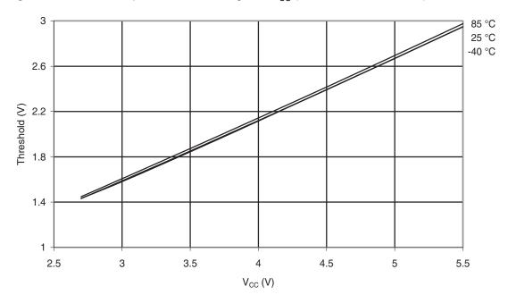
Figure 29-31. I/O Pin Input Threshold Voltage vs.  $V_{\rm CC}$  (VIL, I/O Pin Read as '0')
