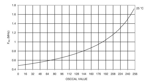
Figure 29-42. Calibrated 1 MHz RC Oscillator Frequency vs. Osccal Value
