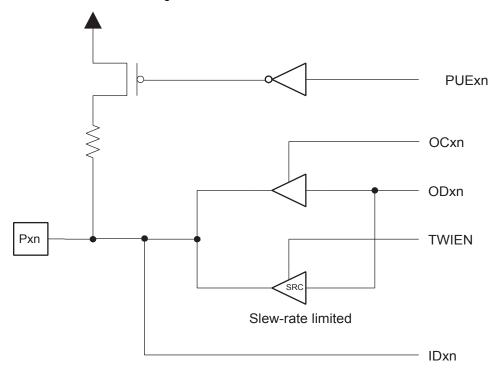
Figure 25-5. Additional Scan Signal for the Two-wire Interface
