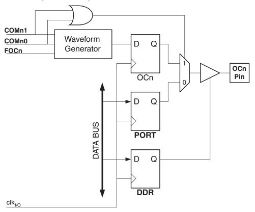
The general I/O port function is overridden by the Output Compare (OC2) from the Waveform Generator if either of the COM21:0 bits are set. However, the OC2 pin direction (input or output) is still controlled by the Data Direction Register (DDR) for the port pin. The Data Direction Register
