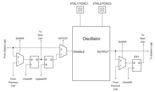
Table 25-3 summaries the scan registers for the external clock pin XTAL1, oscillators with XTAL1/XTAL2 connections as well as 32 kHz Timer Oscillator.
