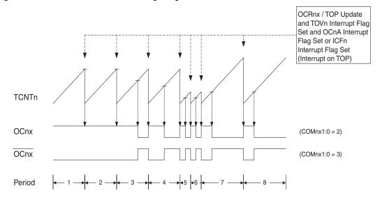
The Timer/Counter Overflow Flag (TOVn) is set each time the counter reaches TOP. In addition the OCnA or ICFn flag is set at the same timer clock cycle as TOVn is set when either OCRnA or ICRn is used for defining the TOP value. If one of the interrupts are enabled, the interrupt handler routine can be used for updating the TOP and compare values.
