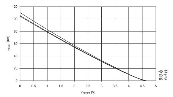
Figure 29-22. Reset Pull-up Resistor Current vs. Reset Pin Voltage ( $V_{CC} = 5V$ )
