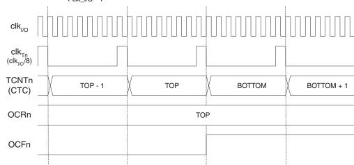
Figure 14-11. Timer/Counter Timing Diagram, Clear Timer on Compare Match Mode, with Prescaler (f<sub>clk |/O</sub>/8)
