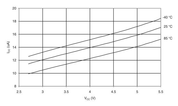
Figure 29-53. ADC Current vs.  $V_{CC}$  (ADC CLK = 50 kHz)
