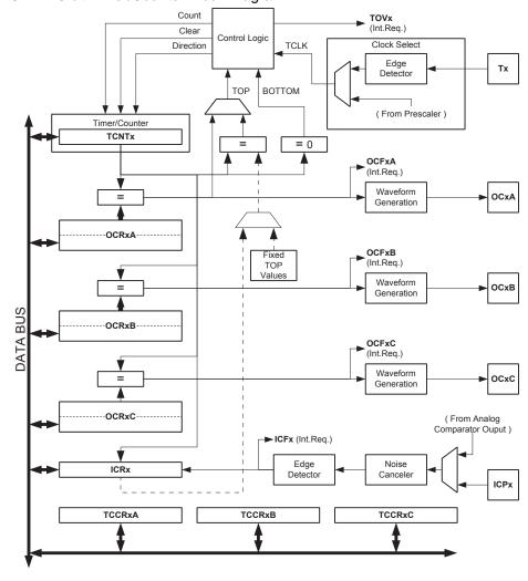
Figure 15-1. 16-bit Timer/Counter Block Diagram<sup>(1)</sup>
