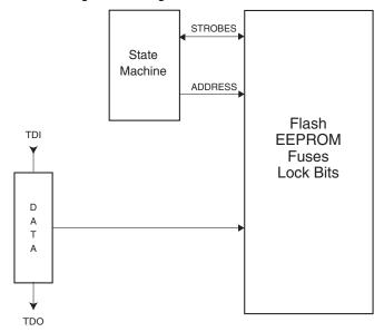
Figure 27-16. Virtual Flash Page Load Register
