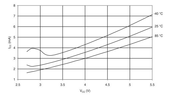
Figure 29-56. Programming Current vs. V<sub>CC</sub>
