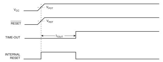
Figure 10-3. MCU Start-up, RESET Extended Externally
