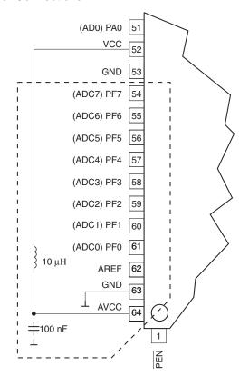
Figure 23-9. ADC Power Connections
