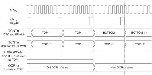
Figure 15-13. Timer/Counter Timing Diagram, with Prescaler ( $f_{clk\_l/O}/8$ )
