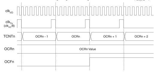
Figure 17-10. Timer/Counter Timing Diagram, Setting of OCF2, with Prescaler (fclk 1/0/8)
