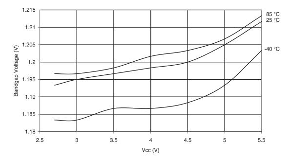
Figure 29-38. Bandgap Voltage vs.  $V_{CC}$
