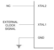
When this clock source is selected, start-up times are determined by the SUT Fuses as shown in Table 8-9.
