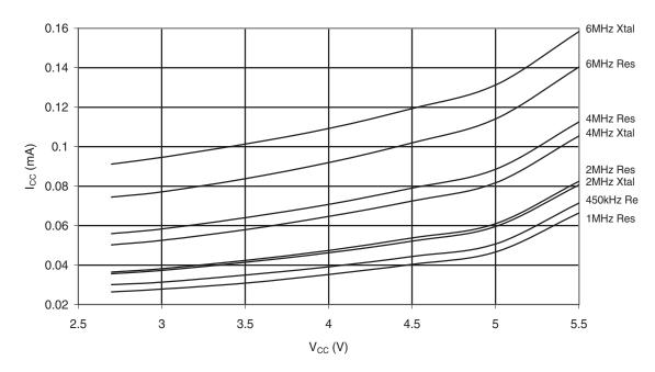
Figure 29-19. Standby Supply Current vs.  $V_{\rm CC}$  (CKOPT Programmed)
