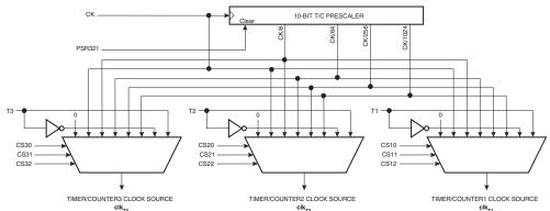
Figure 16-2. Prescaler for Timer/Counter1, Timer/Counter2, and Timer/Counter3<sup>(1)</sup>
