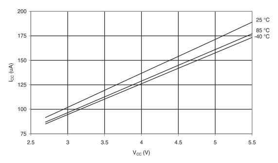
Figure 29-55. Analog Comparator Current vs.  $V_{\rm CC}$
