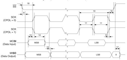
Figure 28-5. SPI Interface Timing Requirements (Slave Mode)
