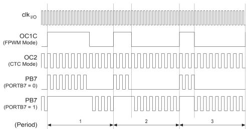
Figure 18-2. Output Compare Modulator, Timing Diagram
