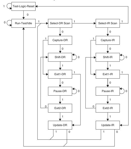
Figure 24-2. TAP Controller State Diagram
