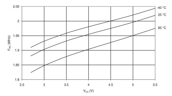
Figure 29-44. Calibrated 2 MHz RC Oscillator Frequency vs.  $V_{\rm CC}$
