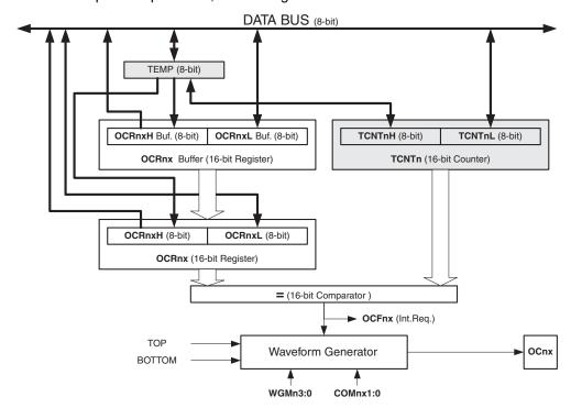
Figure 15-4. Output Compare Unit, Block Diagram
