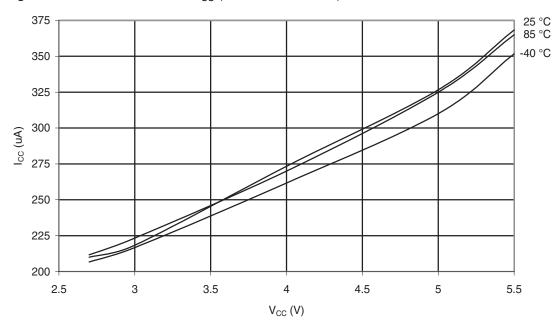
Figure 29-54. Aref Current vs.  $V_{\text{CC}}$
