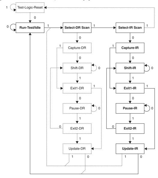
Figure 27-12. State Machine Sequence for Changing the Instruction Word
