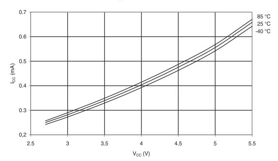
Figure 29-10. Idle Supply Current vs.  $V_{CC}$  (Internal RC Oscillator, 1 MHz)
