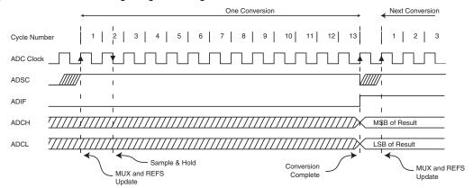
Figure 23-6. ADC Timing Diagram, Auto Triggered Conversion
