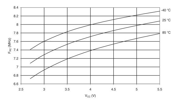
Figure 29-50. Calibrated 8 MHz RC Oscillator Frequency vs.  $V_{\rm CC}$
