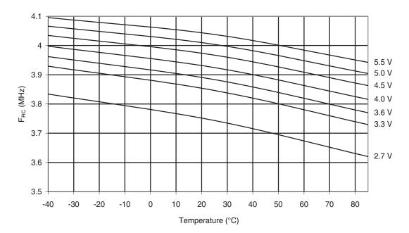
Figure 29-46. Calibrated 4 MHz RC Oscillator Frequency vs. Temperature
