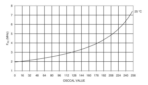
Figure 29-48. Calibrated 4 MHz RC Oscillator Frequency vs. Osccal Value
