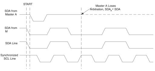
Figure 21-9. Arbitration between Two Masters
