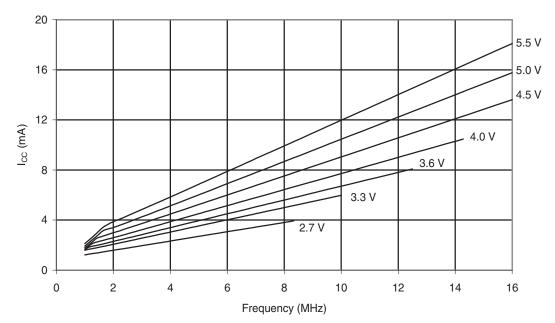
Figure 29-2. Active Supply Current vs. Frequency (1 - 16 MHz)
