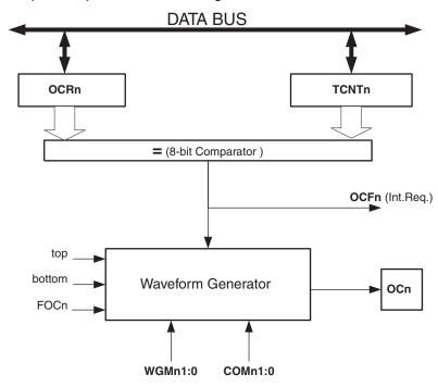
Figure 17-3. Output Compare Unit, Block Diagram
