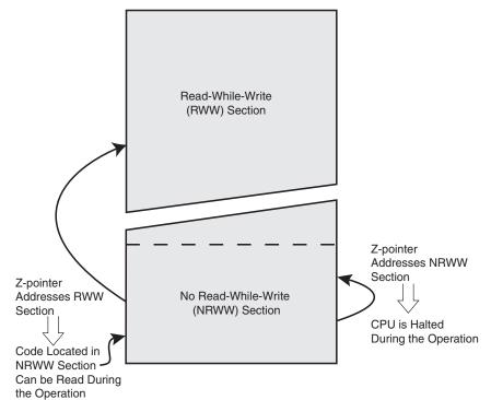
Figure 26-1. Read-While-Write vs. No Read-While-Write
