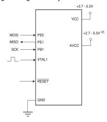
Note: 1. If the device is clocked by the internal Oscillator, it is no need to connect a clock source to the XTAL1 pin.
