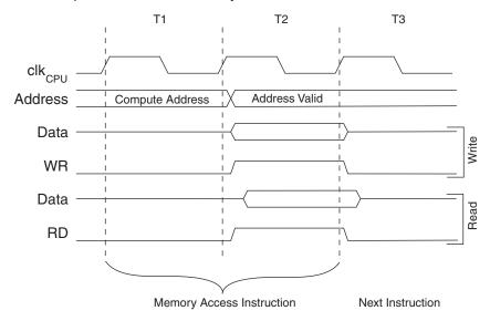
Figure 7-3. On-chip Data SRAM Access Cycles
