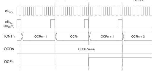
Figure 14-11 shows the setting of OCF0 and the clearing of TCNT0 in CTC mode.
