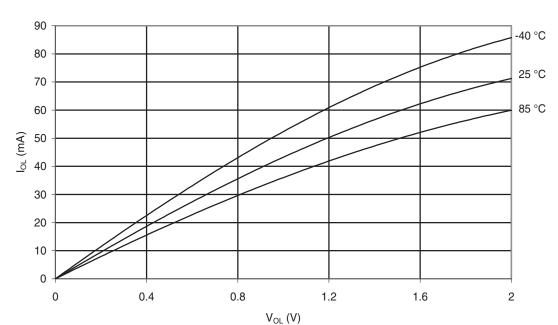
Figure 29-28. I/O Pin Sink Current vs. Output Voltage ( $V_{CC} = 5V$ )
