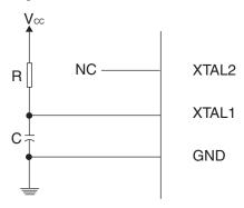
The Oscillator can operate in four different modes, each optimized for a specific frequency range. The operating mode is selected by the fuses CKSEL3:0 as shown in Table 8-5.
