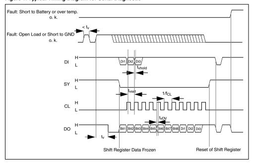
Figure 2. Serial Interface Error Coding
