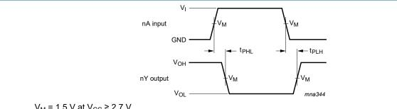
$V_M = 1.5 \text{ V at } V_{CC} \ge 2.7 \text{ V}$
