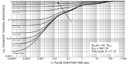
Fig. 12 Transient Thermal Resistance
