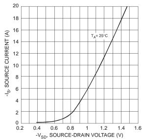
Fig. 20 Diode Forward Voltage vs. Current
