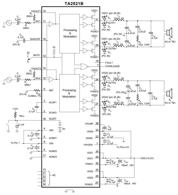
Note: Analog and Digital/Power Grounds must be connected locally at the TA2021
