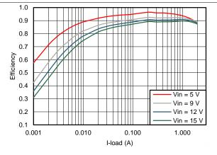
Figure 11. TPS562201  $V_{OUT}$  = 1.8 V Efficiency, L = 2.2  $\mu H$
