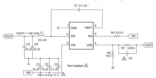
Figure 19. TPS562201 and TPS562208 1.05-V/2-A Reference Design
