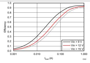
Figure 17. TPS562208  $V_{OUT}$  = 3.3 V Efficiency, L = 2.2  $\mu$ H Figure 17. TPS562208  $V_{OUT}$  = 3.3 V Efficiency, L = 2.2  $\mu$ H
