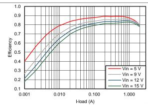
Figure 9. TPS562201  $V_{OUT}$  = 1.05 V Efficiency, L = 2.2  $\mu$ H
