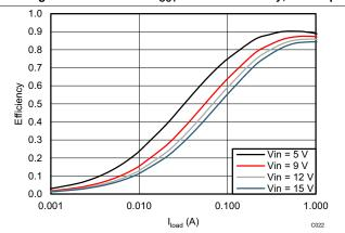
Figure 15. TPS562208  $V_{OUT}$  = 1.5 V Efficiency, L = 2.2  $\mu H$
