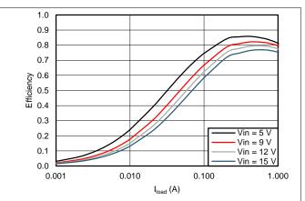
Figure 13. TPS562201  $V_{OUT}$  = 5 V Efficiency, L = 3.3  $\mu H$
