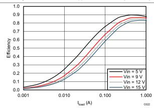
Figure 14. TPS562208  $V_{OUT}$  = 1.05 V Efficiency, L = 2.2  $\mu H$
