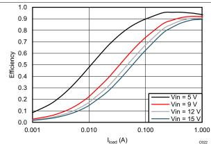
Figure 16. TPS562208  $V_{OUT}$  = 1.8 V Efficiency, L = 2.2  $\mu H$
