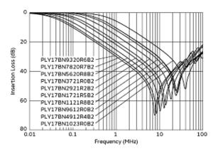
Common Mode Insertion Loss-Frequency Characteristics
