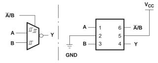
Figure 1. 2-to-1 Data Selector With Inverted Output
