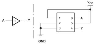
Figure 6. Noninverted Buffer
