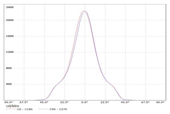
Luminaire: Ledil Oy CN12639\_LENINA-M (Cree CXA20 698Im @ 250mA) Efficiency=85% Lamps: 1 x Cree CXA20 698Im @ 250mA
