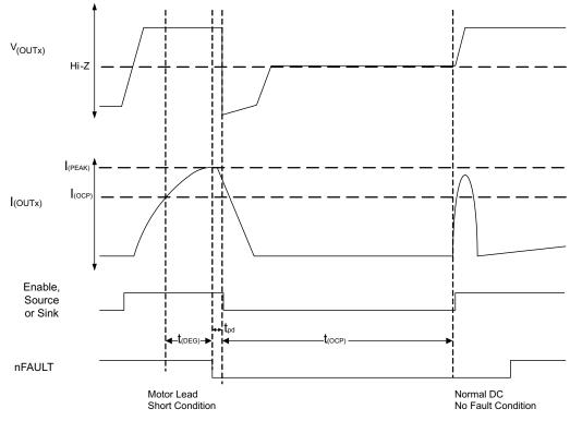
Figure 7. Overcurrent Control Timing
