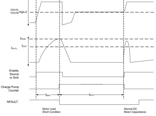
Figure 2. Overcurrent Control Timing
