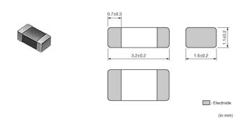
1.The chip ferrite beads BLM series is designed to function nearly as a resistor at noise frequencies, which greatly reduces the possibility of resonance and leaves signal wave forms undistorted. BLM series is effective in circuits without stable ground lines because BLM series does not need a connection to ground.
