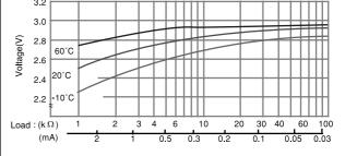
Capacity vs. load resistance
