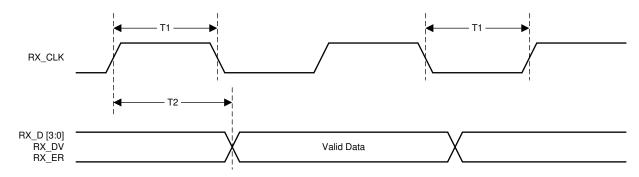
Figure 6-5. 10-Mbps MII Receive Timing
