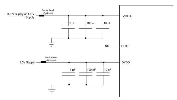
Figure 9-2. DP83TD510E Dual Supply Power Supply Decoupling Recommendation
