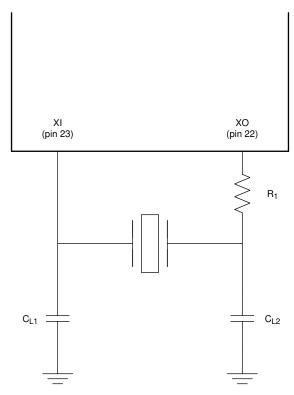
Figure 8-4. Crystal Oscillator Circuit
