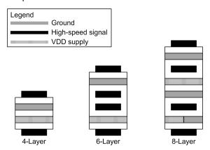
Figure 10-3. Recommended Layer Stack-Up
