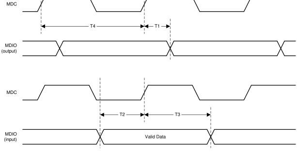
Figure 6-3. Serial Management Timing
