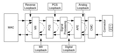
Figure 7-8. Loopback Test Modes
