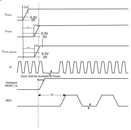
Figure 6-1. Power-Up Timing
