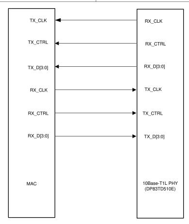
Figure 7-7. RGMII Signalling
