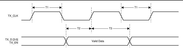
Figure 6-4. 10-Mbps MII Transmit Timing
