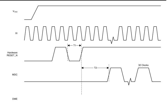
Figure 6-2. Reset Timing
