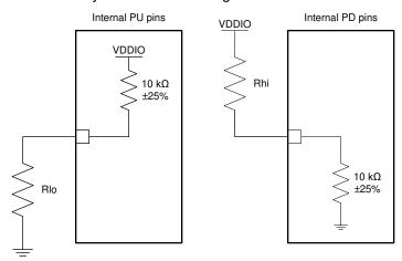
Figure 7-10. Strap Circuit
