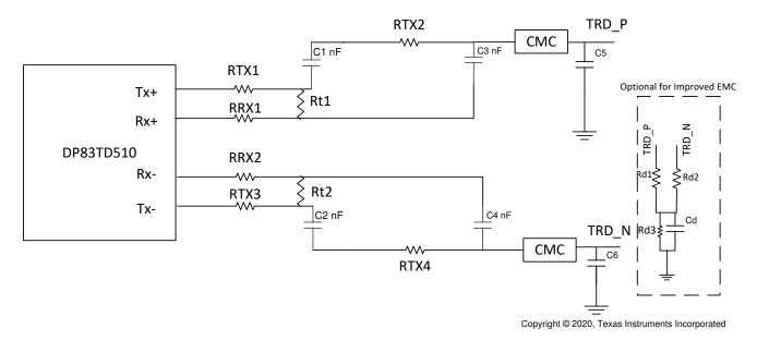
Figure 8-2. Termination Circuit for Intrinsic Safe Applications
