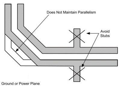
Figure 10-1. Differential Signal Traces
