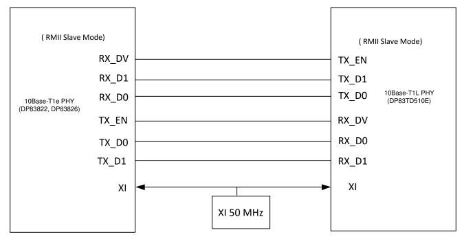
Figure 7-3. Mediaconvertor using RMII MAC interface
