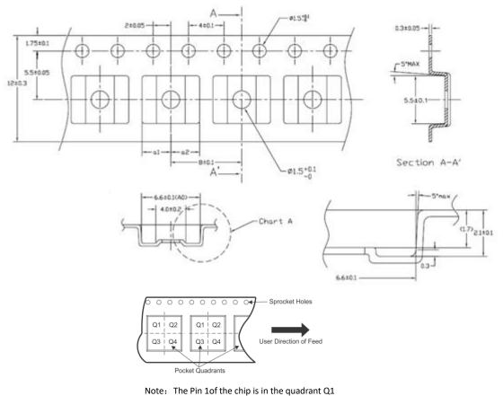
Figure 26. 8-Lead Narrow Body SOIC [NB SOIC-8] Reel Information-dimension unit(mm)
