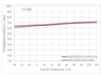
Figure 11. tphl1-2 Propagation Delay vs Free-Air Temperature
