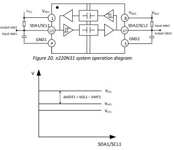
Figure 21.  $\pi$ 220N31/ $\pi$ 221N31 side 1 voltage Diagram
