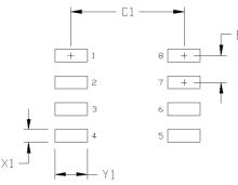
Figure 24.8-Lead Narrow Body SOIC [NB SOIC-8] Land Pattern
