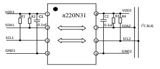
Figure 2. *π*220N31 Typical Application Circuit
