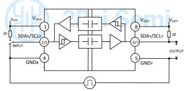
Figure 19. Common-Mode Transient Immunity Test Circuit
