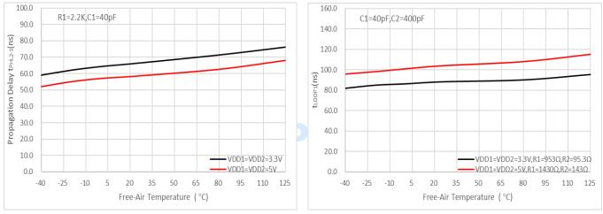
Figure15. tphl2-1 Propagation Delay vs Free-Air Temperature
