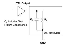
Figure 1. TTL Output AC Test Loading Condition
