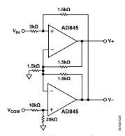
Figure 42. Single-Ended-to-Differential Configuration with the AD845
