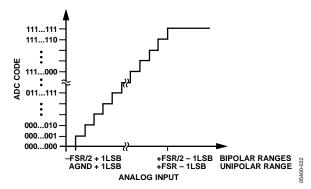
Figure 28. Straight Binary Transfer Characteristic
