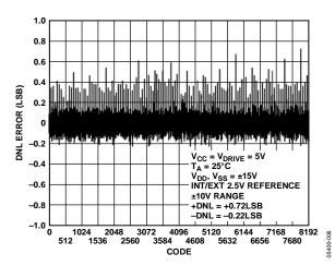
Figure 6. Typical DNL True Differential Mode
