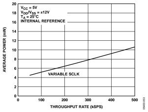
Figure 50. Power vs. Throughput Rate with 5 V Vcc
