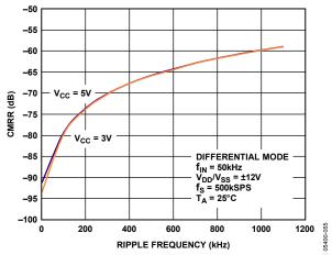
Figure 17. CMRR vs. Common-Mode Ripple Frequency
