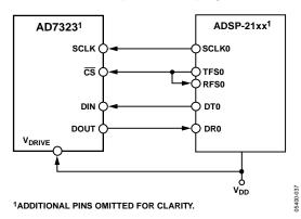
Figure 52. Interfacing the AD7323 to the ADSP-21xx
