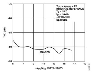
Figure 31. THD vs. ±V<sub>DD</sub>/V<sub>SS</sub> Supply Voltage at 500 kSPS
