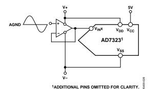
Figure 33. Single-Ended Mode Typical Connection Diagram
