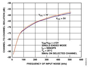
Figure 14. Channel-to-Channel Isolation
