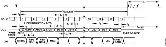
Figure 2. Serial Interface Timing Diagram
