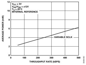
Figure 49. Power vs. Throughput Rate with 3 V Vcc
