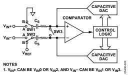
Figure 26. ADC Differential Configuration During Conversion Phase
