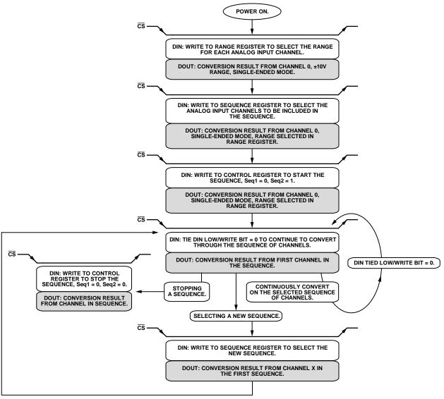
Figure 44. Programmable Sequence Flowchart
