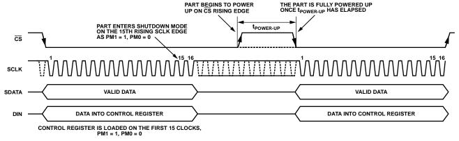
Figure 48. Entering Autoshutdown/Autostandby Mode
