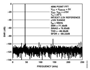
Figure 4. FFT True Differential Mode
