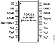
Figure 3. Pin Configuration
