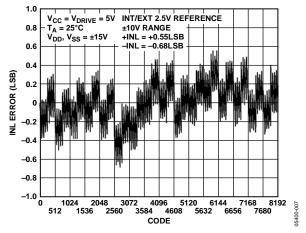
Figure 7. Typical INL True Differential Mode
