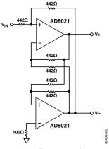
Figure 43. Single-Ended-to-Differential Configuration with the AD8021
