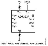
Figure 54. Schottky Diode Connection
