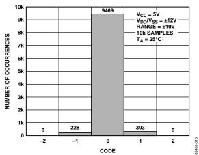
Figure 15. Histogram of Codes, True Differential Mode
