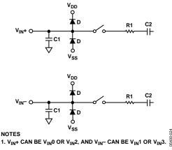
Figure 30. Equivalent Analog Input Circuit (Differential)
