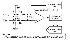
Figure 25. ADC Differential Configuration During Acquisition Phase
