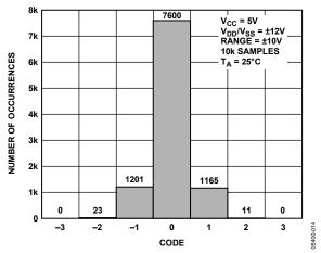
Figure 16. Histogram of Codes, Single-Ended Mode
