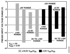
Figure 41. Pseudo Input Range with  $V_{CC} = 3 V$
