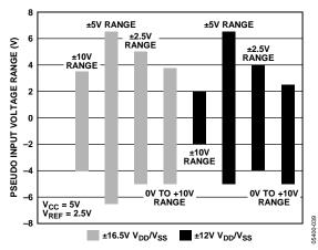
Figure 40. Pseudo Input Range with  $V_{CC} = 5 V$
