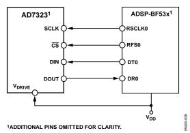
Figure 53. Interfacing the AD7323 to the ADSP-BF53x
