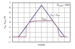
Figure 33. Power-Up and Power-Down Response
