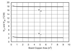
Figure 35.  $\Psi_{\text{JT}}$  and  $\Psi_{\text{JB}}$  vs Board Size
