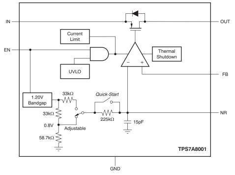
Figure 29. Adjustable Voltage Version
