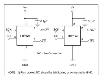
Figure 1. Typical Connections of the TMP121 and TMP123
