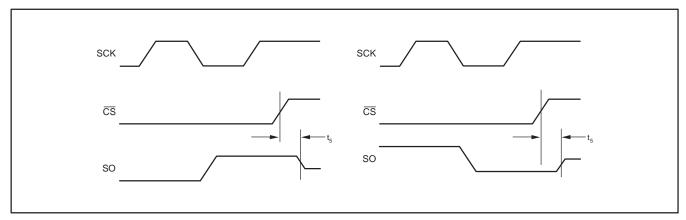
Figure 5. High Impedance Output Timing Diagram
