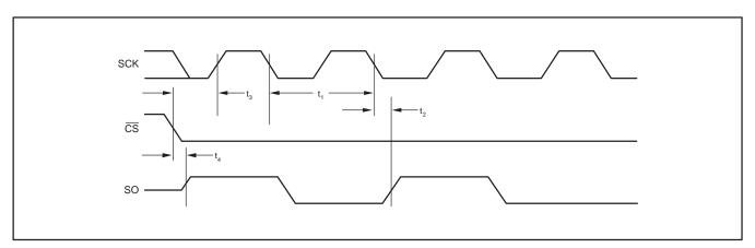
Figure 4. Output Data Timing Diagram
